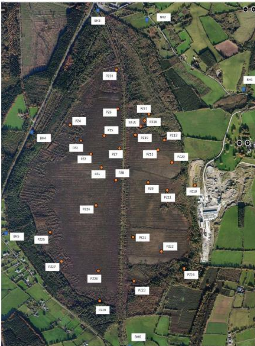
Figure B: Existing Borehole and Piezometer Monitoring Network at Abbeyleix Bog (after Swenson, 2017) 1
